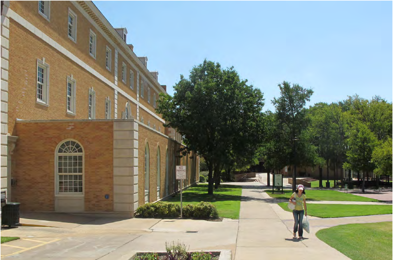
The photo above illustrates how the overall building massing defines the street edge, while the first floor extension helps to define the building entrances and the tall arched windows reveal interior activity to the pedestrians on the sidewalk. The straight line of trees further reinforces the sidewalk space.
